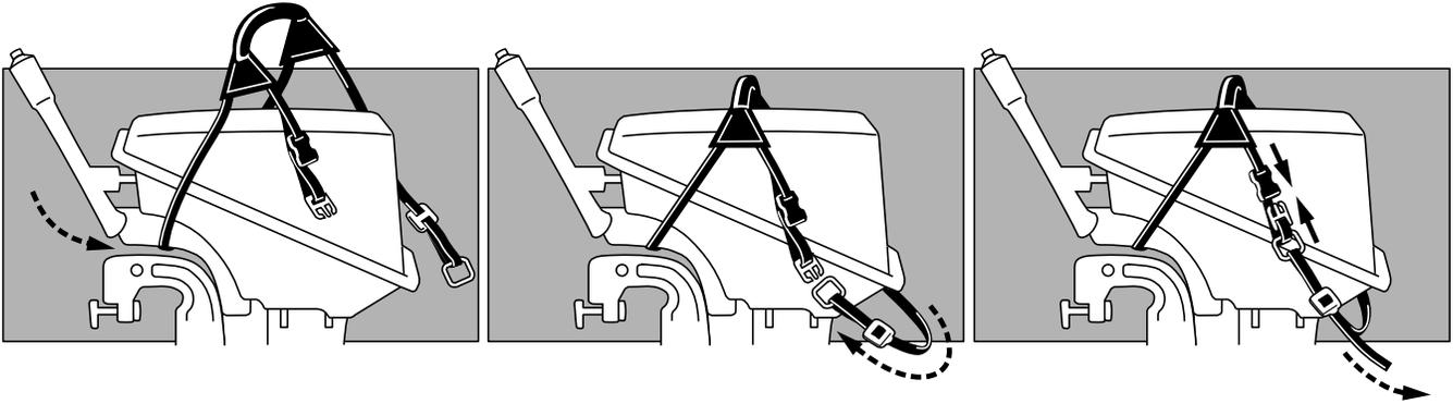
The harness may be installed with buckle on either side of motor. The webbing is one continuous piece; pulling on one side will tension the other side.
