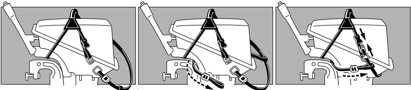
Release the attachment buckle. Slide the security strap's small loop onto the harness webbing in back of motor.
